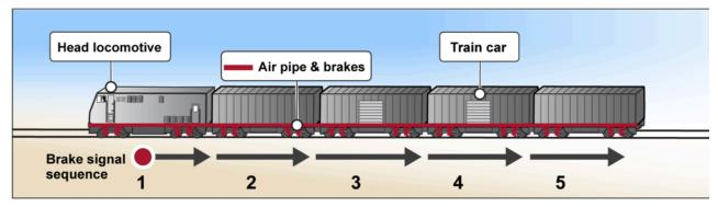
A train uses an air braking system developed in the 1800s, and the longer the train, the harder it is to maintain adequate air in the system.
