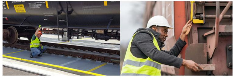
Required brake tests take longer on a long train. Some brake tests require the inspection of every car, and walking a 3-mile-long train to the end and back is 6 miles. Add to that a portable radio that fails to transmit, and the result is substantial train delay.
