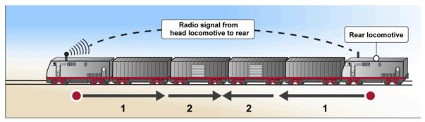
Train operations require that the crew in the lead locomotive maintain constant communications with the rear locomotives or the device on the rear car of the train. When these communications fail, the train is restricted to 30mph, and in some instances, the train is required to stop. The longer the train, the more these communications fail. This loss of communications is very common when trains go around curves or go over the tops of mountains.
