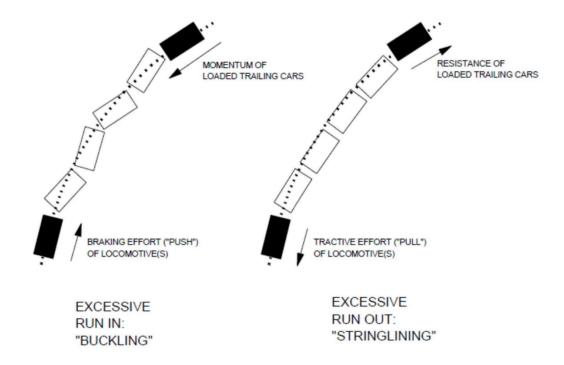
Longer trains result in more derailments per train mile. These derailments will have more severe impacts (cars derailed, products released, and potential evacuations). Regarding manifest trains (mixed rail cars) and distributed power, the potential for derailment forces above those previously projected.
